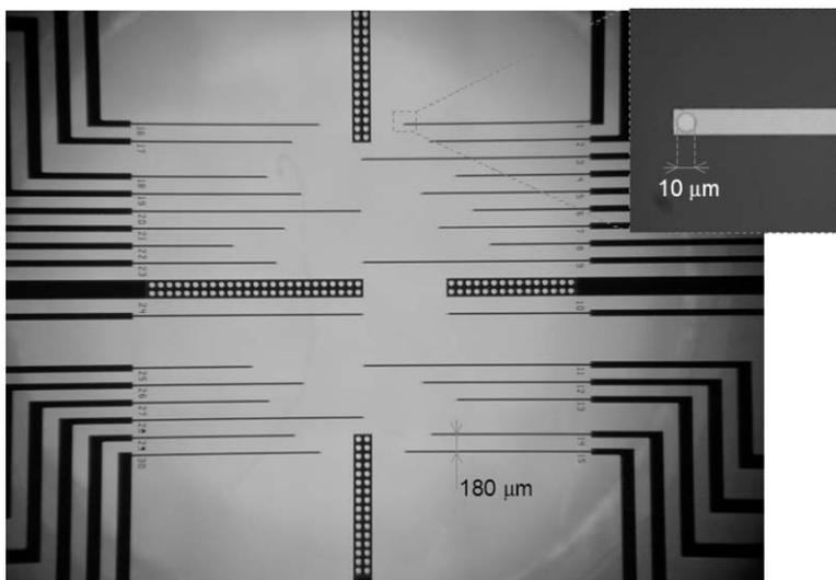
**Figure 4.** Example of an array of 30 planar microelectrodes, microfabricated on a silicon substrate, designed and developed at the Institute of Microtechnology, University of Neuchatel, Switzerland (picture kindly provided by L. Berdondini).
